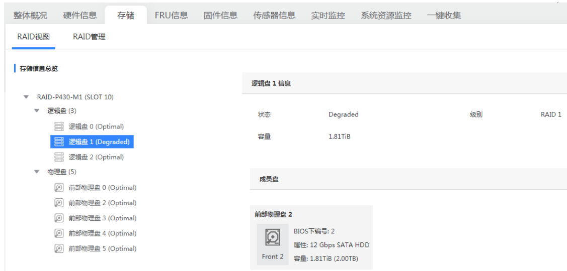
图7-61 逻辑盘状态显示为 Degraded
